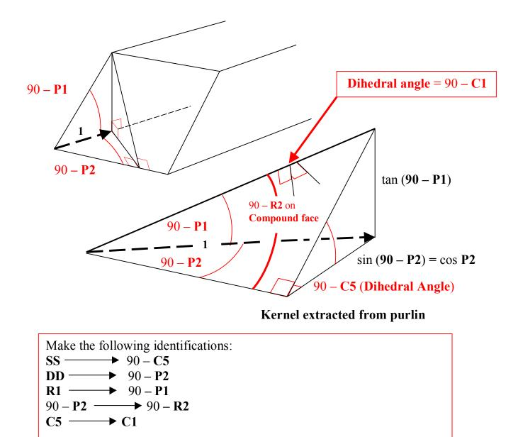
The values of two of the angles are known; 90 - C5 is the dihedral angle between the face lying on the roof plane and the face which meets the side of the hip rafter, and 90 - P2 is the required miter angle on the roof plane. The remaining angles may now be resolved.
