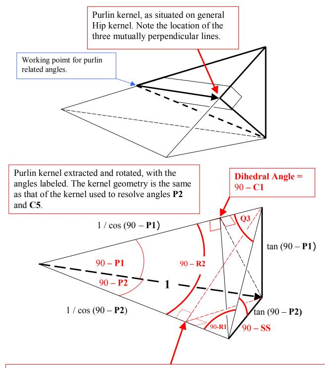
The kernel may be divided along the lines of dihedral angle 90 - C5, resulting in two kernels: the kernel of Common rafter angles, and a kernel the same as that extracted from the stick. However, this kernel will be analyzed as it sits, to demonstrate that there is more than one method, or one type of geometry, whereby it is possible to obtain angle formulas.
