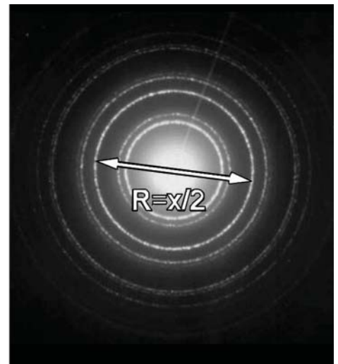
Fig. 4: Electron diffraction pattern from an unknown sample, suspected to be aluminum.
