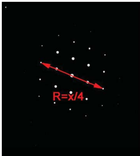
Fig. 2: Electron diffraction pattern from single crystal silicon, with the beam parallel to the [011] zone axis.
